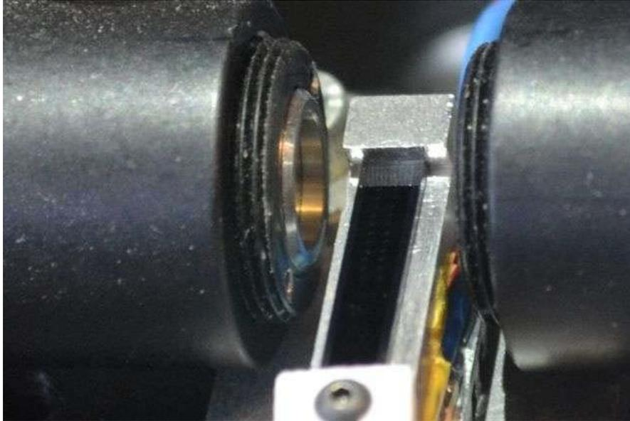
The optical clock developed by UCLA Engineering researchers is the small black strip between the two black cylinders.
