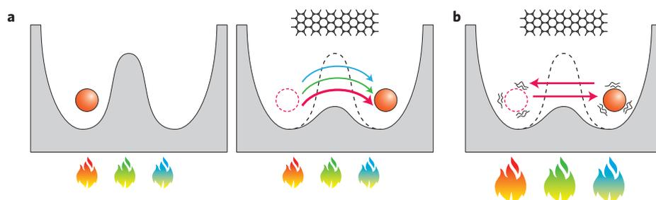
**Figure 1** | Double-well model of excitation-dependent nonlinear optical phenomena in a graphene–silicon hybrid system. **a**, A graphene-on-silicon photonic crystal cavity reduces the potential barrier to facilitate optical bistability during heating. The colours of each flame represent the detuned wavelengths of the input laser. **b**, Increased heating power induces regenerative oscillation between the two potential wells.
